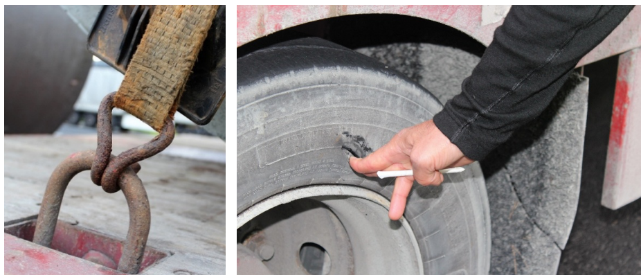
Image 5: Cargo securing equipment and truck tire lacking maintenance. Photo: Reidar Mikkelsen.
